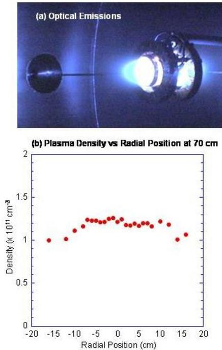
**Figure 15: Plasma density as distance increases from the HPH with no nozzles [1]**
