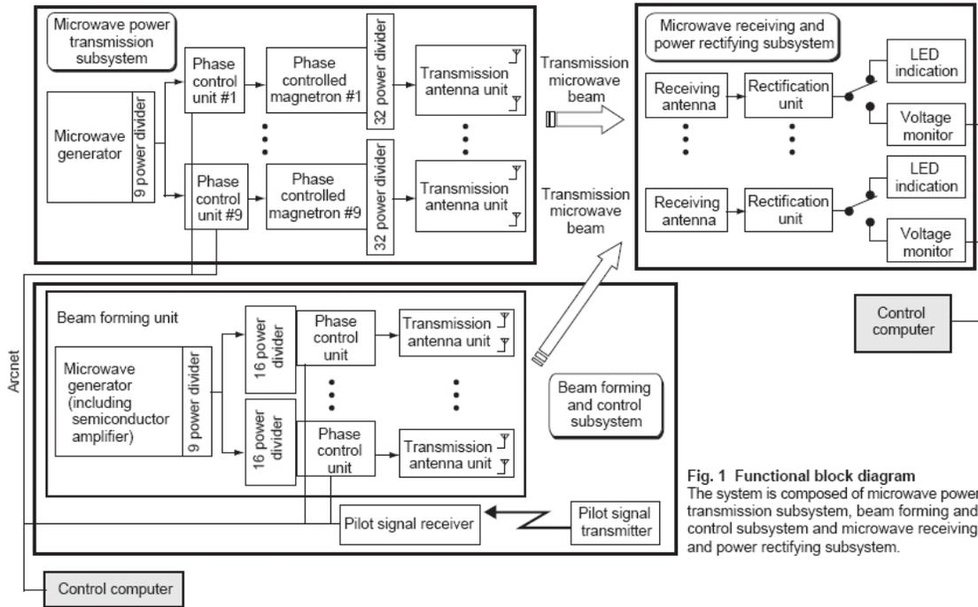
**Figure 1: Microwave system block diagram [2]**
