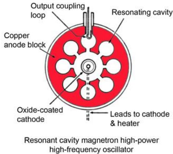
**Figure 2: Magnetron Cross Section [3]**
