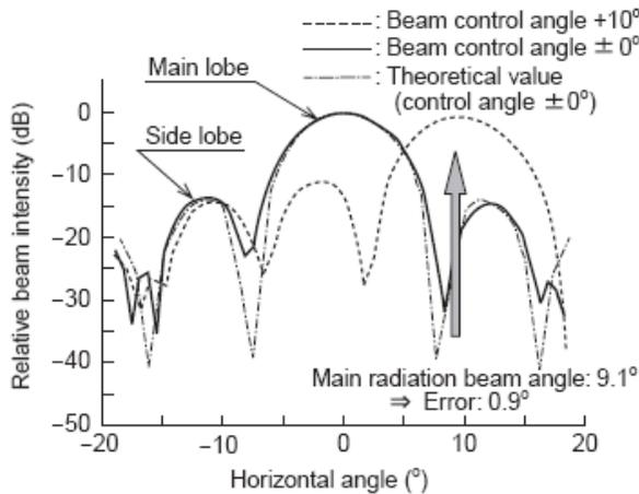
**Figure 6: The plot shows the beam power received relative to the receiver angle. [2]**
