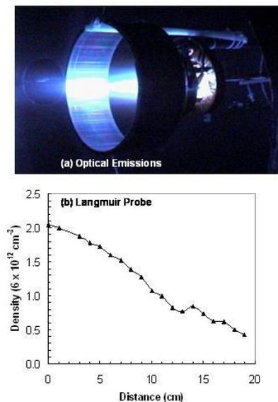
**Figure 16: Plasma flow with the addition of one magnetic nozzle**
