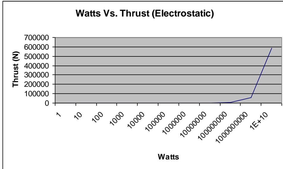
**Figure 8: Thrust vs. Watts for an electrostatic engine**
