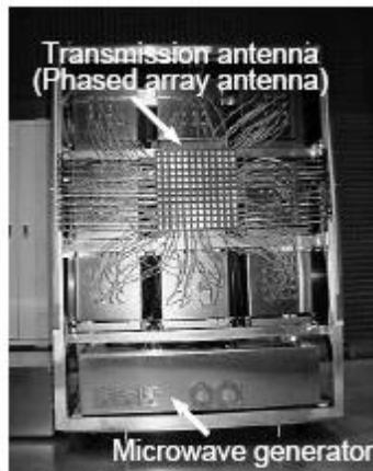
**Figure 4: Beam Forming and Control subsystem**
