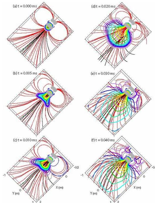
**Figure 12: Plasma propagation with out magnetic nozzles [1]**
