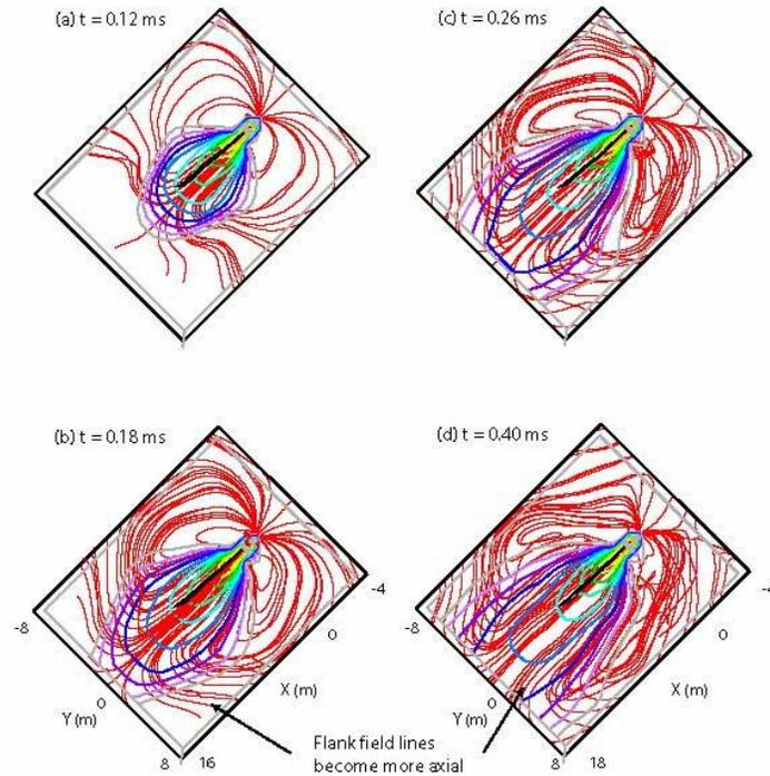
**Figure 14: Plasma propagation with the addition of a second magnetic nozzle [1]**
