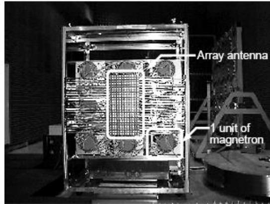
**Figure 3: Microwave Generator and Transmitter Subsystem [2]**
