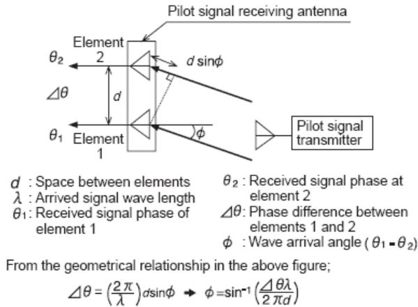
**Figure 5: Receiver Phase Angle Detection [2]**
