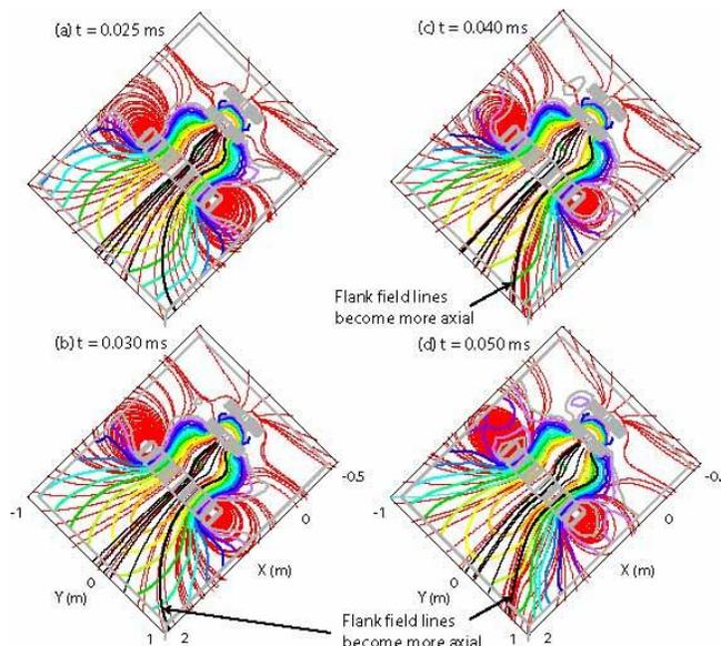
**Figure 13: Plasma propagation with one magnetic nozzle [1]**
