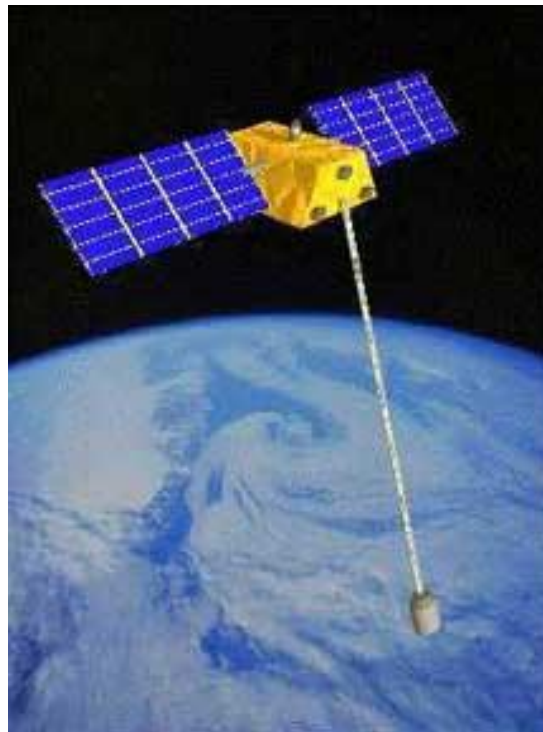
Figure 1. NASA drawing of a satellite utilizing tethered attitude control.
