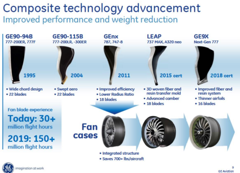
Figure 5. Composite Technology advancement in the GE engines
