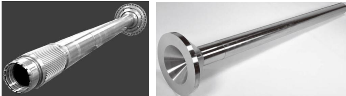
Figure 9. Mid Fan Shaft (Left) and low-pressure turbine shaft (Right) in the GE1014 engine
