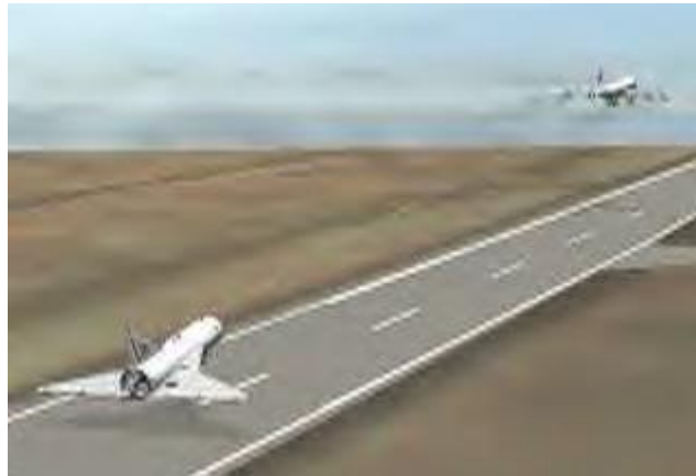
Fig. 4 Astroliner, a towed air launch vehicle. 4
