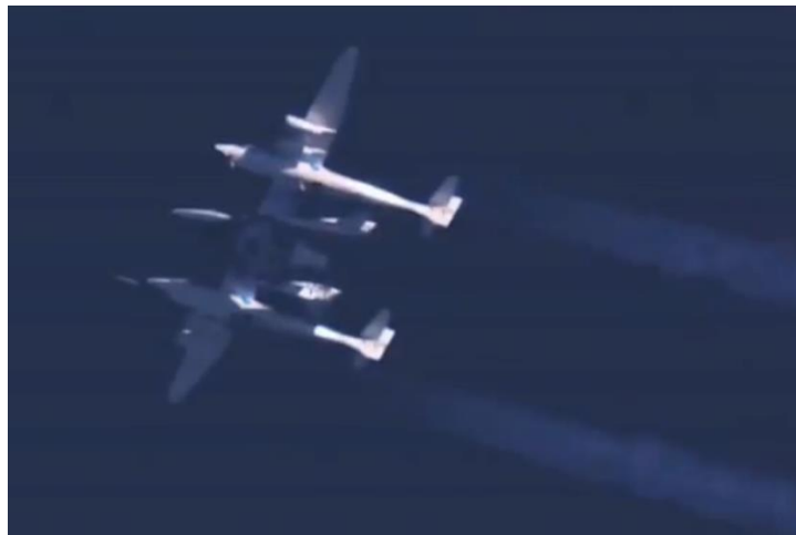
Fig. 3 LauncherOne carried underneath WhiteKnightTwo. 12
