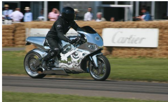
Figure 6: The MTT Superbike uses an M250 turboshaft engine
