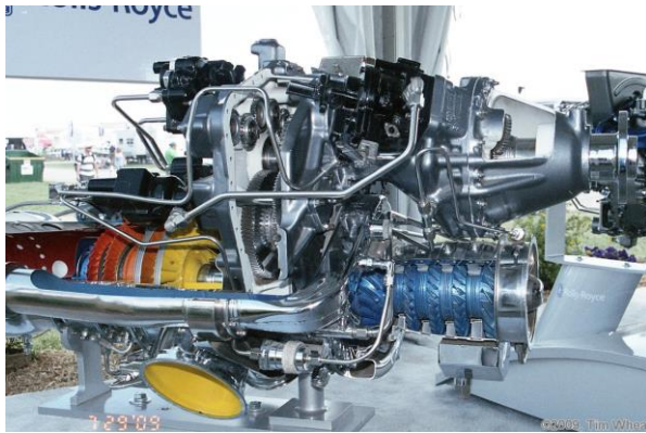
Figure 4: RR M250 turboshaft. Notice the color of paint indicating the temperature of the gases in that section
