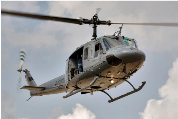
Figure 7: The UH-1 Huey helicopter is powered by a Lycoming T53.
