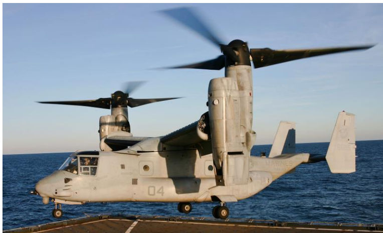
Figure 9: V-22 Osprey uses two T406 turboshafts
