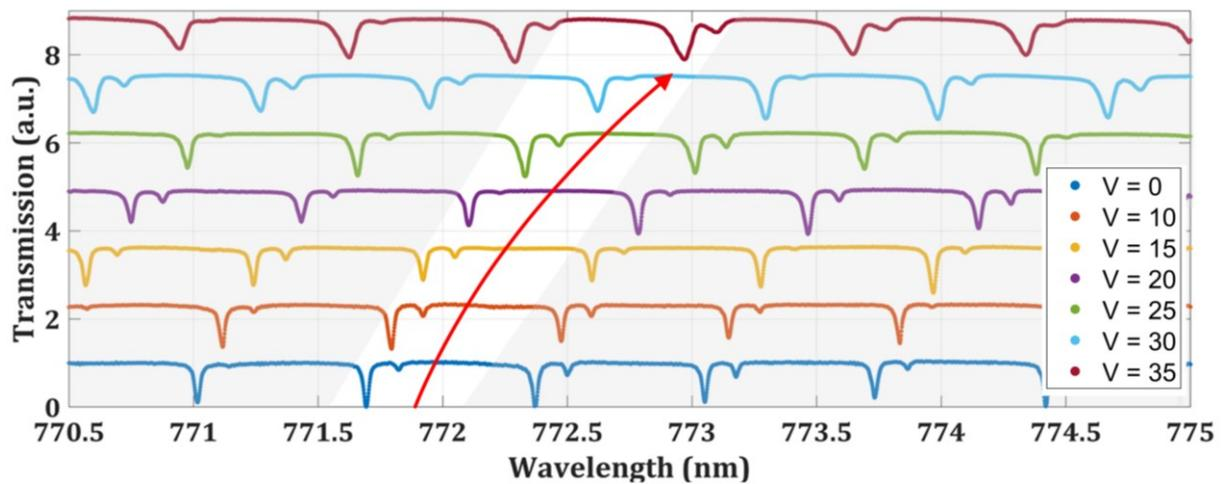
Figure 6: Recorded transmission signal as a function of actuating voltage on a glycerol droplet surrounded by dodecane. The two peaks repeated across the spectra correspond to resonance modes of TM and TE polarization. When a voltage function is applied, the resonance frequency redshifts in agreement with the prediction through the electrowetting equation. Free spectral range is measured at 0.679 nm.
