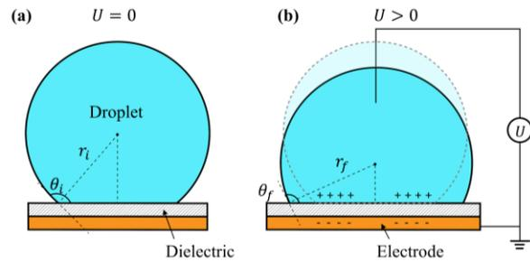
Figure 1: (a) Geometry of a liquid droplet on a dielectric solid surface with an initial contact angle of  $\theta_i$  and a radius of  $r_i$ . (b) Charge buildup on the dielectric surface upon the application of an electric potential. This leads to a decrease in contact angle and an expansion of equatorial radius.
