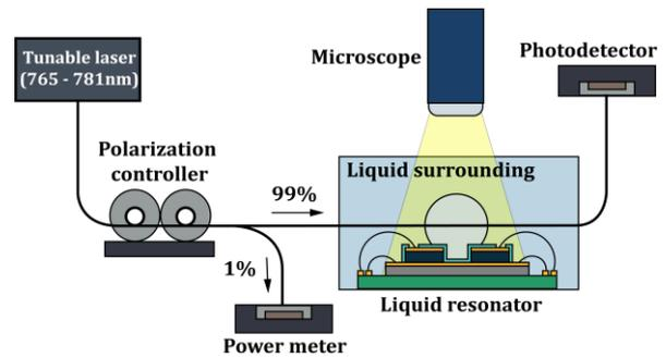
Figure 3: Schematic of the liquid microresonator experimental setup. Light is coupled into the liquid droplet microresonator through a tapered fiber. The tunable laser is swept across a spectral range (770-775 nm). A fast photodetector measures power in the transmission and a power meter monitors the input power.
