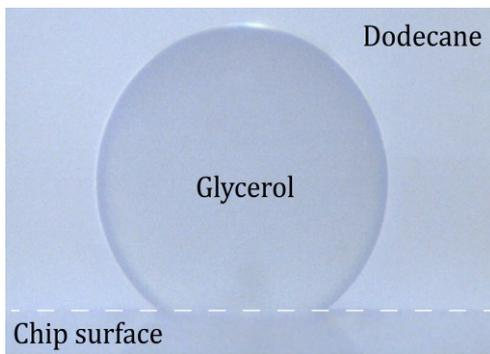
Figure 4: Side view image of a glycerol liquid droplet on the electrowetting chip surrounded by a dodecane bath. Dashed line indicates the surface of the chip. Initial contact angle is measured at  $145.8^\circ$  with a diameter of  $191\ \mu\text{m}$ .
