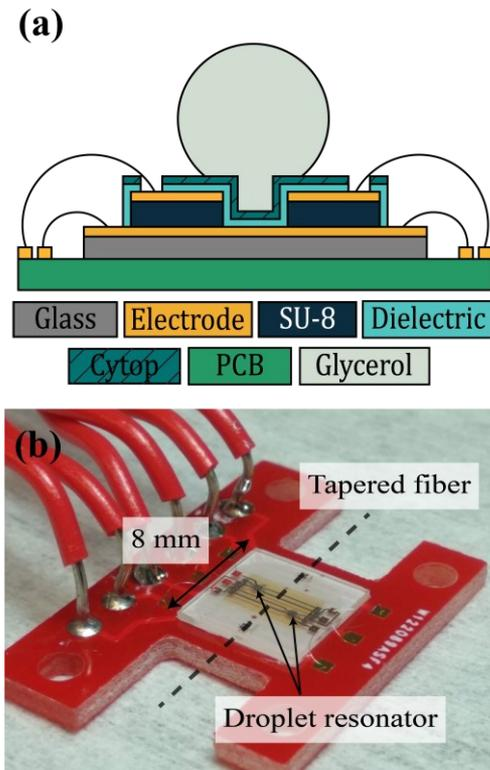
Figure 2: (a) Cross-sectional view of the liquid microresonator chip (b) Assembled device with electrical connections bonded to the external PCB pads. SU-8 wells are situated off-center to allow tapered fiber to couple to each droplet.
