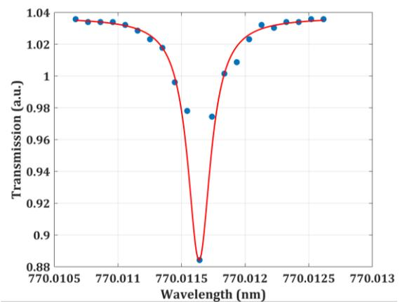
Figure 5: A Q-factor of  $3.5 \times 10^6$  is measured by fitting a Lorentzian function to the resonance peak of the glycerol droplet in hexane system.
