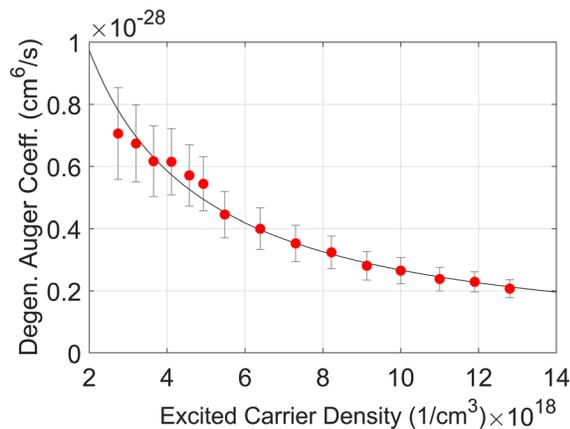
**FIG. 3.** Cubic Auger coefficients of a representative sample measured in a range of nominal excited carrier densities, all above the degenerate limit. The coefficients are fit to Eq. (3), from which we extract a low-carrier-density cubic Auger coefficient  $C_3^0$  for each sample.
