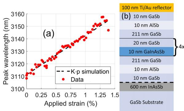
**FIG. 1.** (a) Peak photoluminescence wavelength with applied strain compared to the simulated shift in the bandgap expected for the given applied strain. The bandgap shift is calculated using eight-band  $k \cdot p$  simulations.<sup>17</sup> (b) Sample layer structure. The Ti/Au reflector layer is bonded to either a flexible membrane or inflexible heat sink. The region below the dashed line is etched away prior to the measurement.
