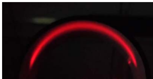
Figure 1. Beam scanning over 180° at 200 Hz, using an electrowetting prism that can be applied to LIDAR.
