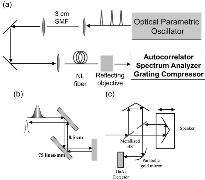
Fig. 5. Experimental setup for (a) supercontinuum generation in highly nonlinear bismuth-oxide fiber, (b) subsequent pulse compression using a grating pair, and (c) broadband autocorrelator.
