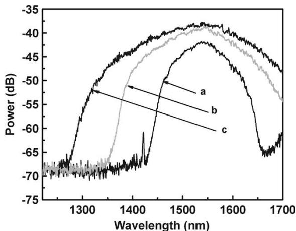
Fig. 9. Spectra as a function of input power produced in a 1-m length of fiber at an input wavelength of 1540 nm. Average input powers and pulse energies were (a) 10 mW/0.12 nJ, (b) 20 mW/0.24 nJ, and (c) 34 mW/0.41 nJ.
