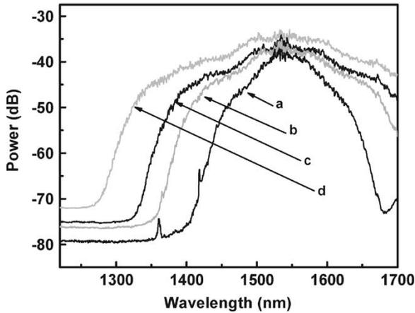
Fig. 6. Spectra as a function of input power produced in a 2-cm length of fiber at an input wavelength of 1540 nm. Average powers exiting the fiber were (a) 7 mW, (b) 14 mW, (c) 21.4 mW, and (d) 32 mW. Insufficient attenuation of cladding modes causes the interference apparent at the center of the spectra.
