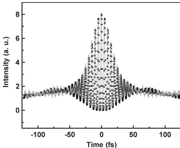
Fig. 8. Interferometric autocorrelation of compressed pulses produced with 2 cm of fiber and a grating compressor. The PICASO phase-retrieval algorithm was used to fit the data, and a pulsewidth of 25 fs is extracted. (Solid line: experimental result, black dots: retrieved autocorrelation).
