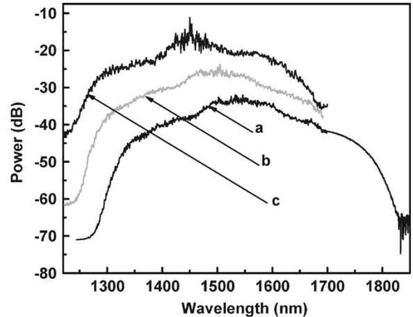
Fig. 7. Spectra as a function of input excitation wavelength from a 2-cm fiber at an average input power of 32 mW. Input wavelengths were (a) 1540 nm, (b) 1500 nm, and (c) 1450 nm. An optical spectrum analyzer was used for the spectra up to 1700 nm, and a spectrometer was used from 1700–1900 nm. The spectra are vertically offset for ease of viewing.
