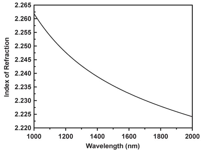
Fig. 2. Index of refraction versus wavelength for bismuth-oxide glass.
