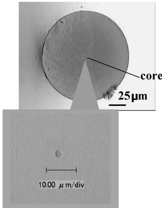
Fig. 1. Cross-section of highly nonlinear bismuth-oxide fiber.
