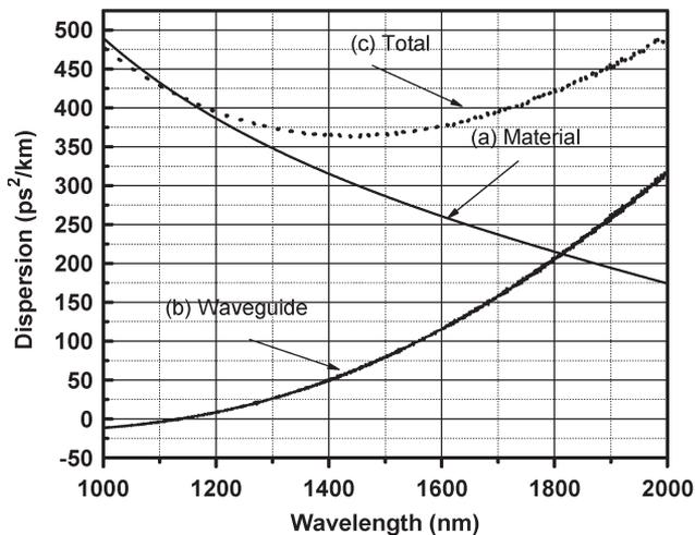
Fig. 3. Dispersion as function of wavelength for (a) bismuth-oxide glass (material), (b) waveguide, and (c) total dispersion of the fiber.
