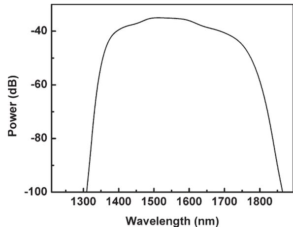
Fig. 4. Simulation results for supercontinuum generation in 2 cm of bismuth-oxide fiber with 2.6 kW of peak power incident at 1540 nm.
