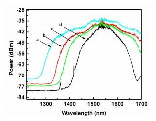
Fig. 1. Spectra from a 2-cm piece of fiber generated by 1540-nm excitation at average powers exiting the fiber of: a) 32 mW b) 21.4 mW c) 14 mW d) 7 mW. The interference at the center of the spectra is due to insufficient attenuation of cladding modes.
