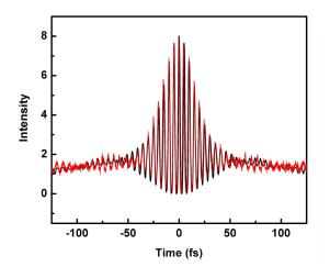
Fig. 3. Fringe resolved autocorrelation of 25-fs pulses generated from 2 cm of fiber with 150-fs input pulses at 1540 nm. The pulse is fitted with the Picaso phase retrieval algorithm.
