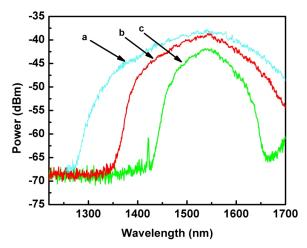
Fig. 4. Supercontinuum spectra from 1 m of highly nonlinear bismuth oxide fiber generated by 1540-nm excitation at average powers exiting the fiber of: a) 34 mW b) 20 mW c) 10 mW.
