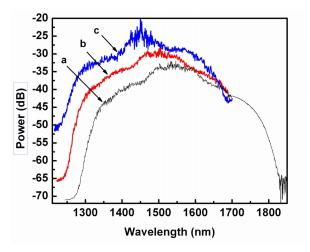
Fig. 2. Spectra from a 2-cm length of fiber of input wavelengths of: a) 1540 nm b) 1500 nm c) 1450 nm. The spectra were taken up to 1700 nm with an optical spectrum analyzer, and the measurement from 1700 - 1900 nm was taken with a spectrometer. The spectra were all taken for comparable powers and are vertically offset for ease of viewing.
