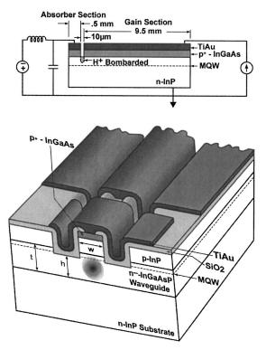
Fig. 1. Schematic of multisection slab-coupled optical waveguide laser device with waveguide dimensions:  $w = 5.8 \ \mu \text{m}, t = 4.9 \ \mu \text{m}, \text{ and } h = 4.5 \ \mu \text{m}.$
