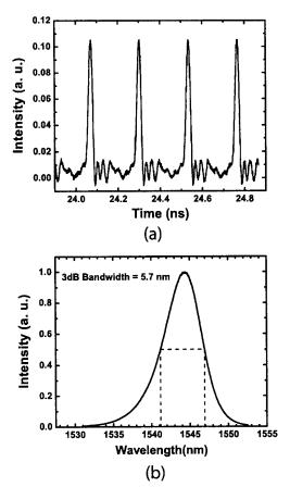
Fig. 2. (a) Sampling scope trace of pulse train. (b) Optical spectrum of mode-locked device measured with 0.1 nm of resolution.
