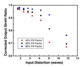
Fig. 4. (Color online) Output Strehl ratio versus input distortion in waves for a variety of different fill factors for a lens and prism array: 40% fill factor (red triangles), 58% fill factor (black circles), and 80% fill factor (blue squares). Simulation includes tip-tilt, curvature, and piston compensation. The arrays consist of 19 elements that are 2 mm in diameter and are filled with water and air.
