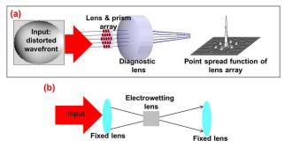
Fig. 3. (Color online) Setups for simulations. (a) A distorted wave is input to a 19-element lens and prism array. A diagnostic lens focuses the resulting corrected wavefront, and the PSF of the lens array and Strehl ratio are measured. (b) Light is input to a telescope with an electrowetting element placed at the focus. This setup is used to evaluate the piston-adjustment capabilities of the electrowetting lens.
