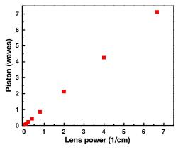
Fig. 6. (Color online) Effect of focal length tuning on piston compensation for 1 mm diameter lenses with 2 mm thickness containing equal quantities of oil and water. As the lens curvature becomes flatter (corresponding to longer focal length), larger changes in focal length are needed to produce piston delay.
