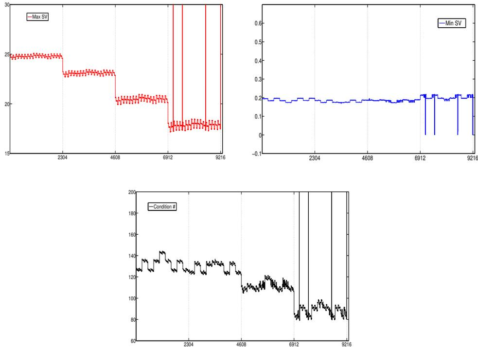
FIG. 4.2. The top two figures show the maxima and minima singular values of all the 9216 systems with the two-level hybrid preconditioner, the bottom figure shows the condition numbers of all the 9216 systems with the two-level hybrid preconditioner.
