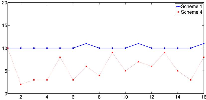
FIG. 5.4. One-level RAS preconditioning, comparison of numbers of iterations for Scheme 1 and 4 in the bad group
