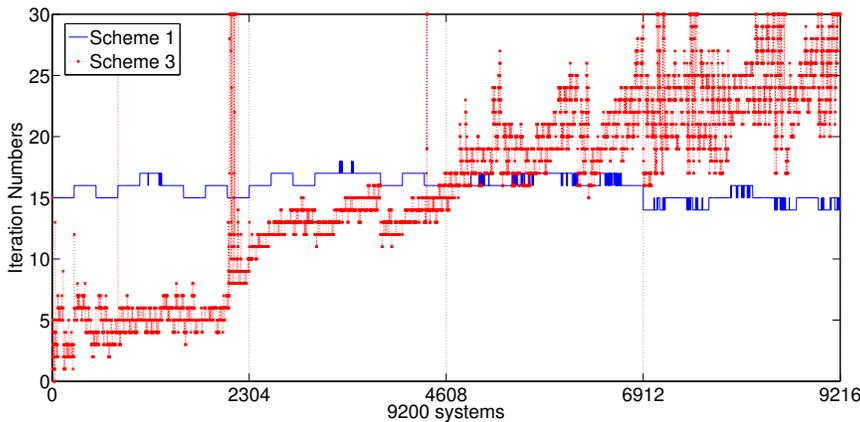
FIG. 5.6. *Two-level hybrid preconditioning, comparison of numbers of iterations for Scheme 1 and 3*
