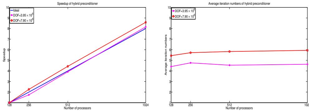
FIG. 5.9. Speedup and average numbers of iterations of two-level hybrid preconditioner
