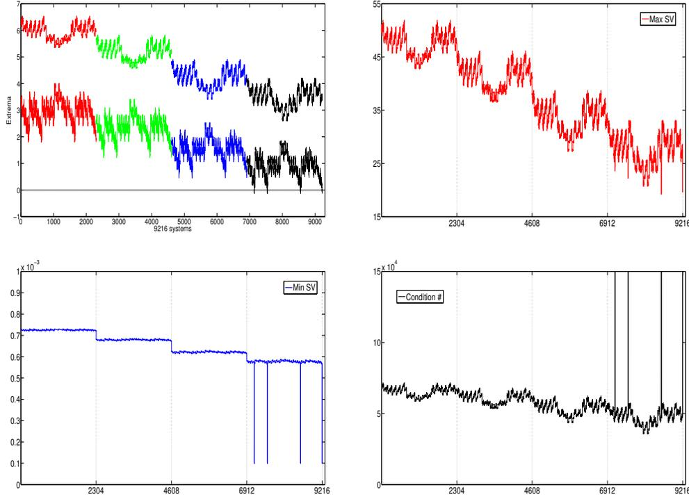
FIG. 4.1. The top left figure shows the maxima and minima of the diffusion coefficients  $a_{M,i}(x)$  for all the 9216 systems. The top right and bottom left figures show the maxima and minima singular values of all the 9216 systems without any preconditioning. The bottom right figure shows the condition numbers of all the 9216 systems without any preconditioning.
