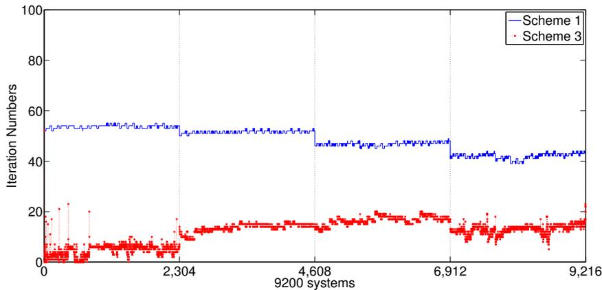
FIG. 5.2. *One-level RAS preconditioning, comparison of numbers of iterations for Scheme 1 and 3*
