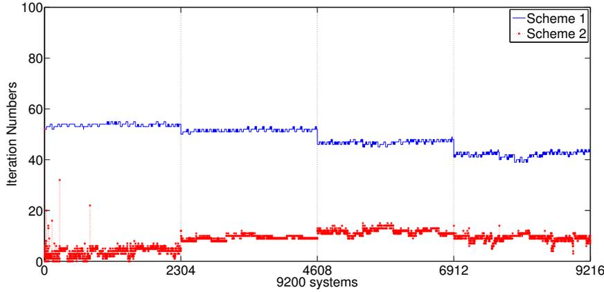
FIG. 5.1. One-level RAS preconditioning, comparison of numbers of iterations for Scheme 1 and 2
