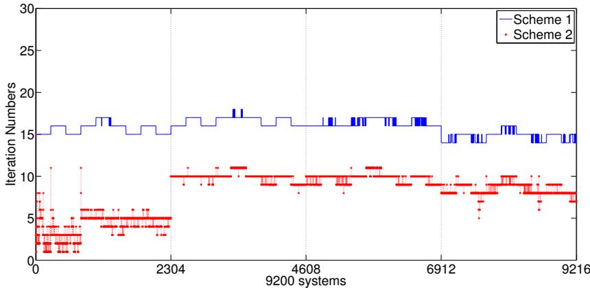
FIG. 5.5. Two-level hybrid preconditioning, comparison of numbers of iterations for Scheme 1 and 2
