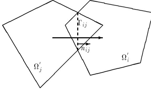
Figure 1: The term  $T_i T_j$  is kept in the Schwarz polynomial only if the flow goes from  $\Omega'_j$  to  $\Omega'_i$ .
