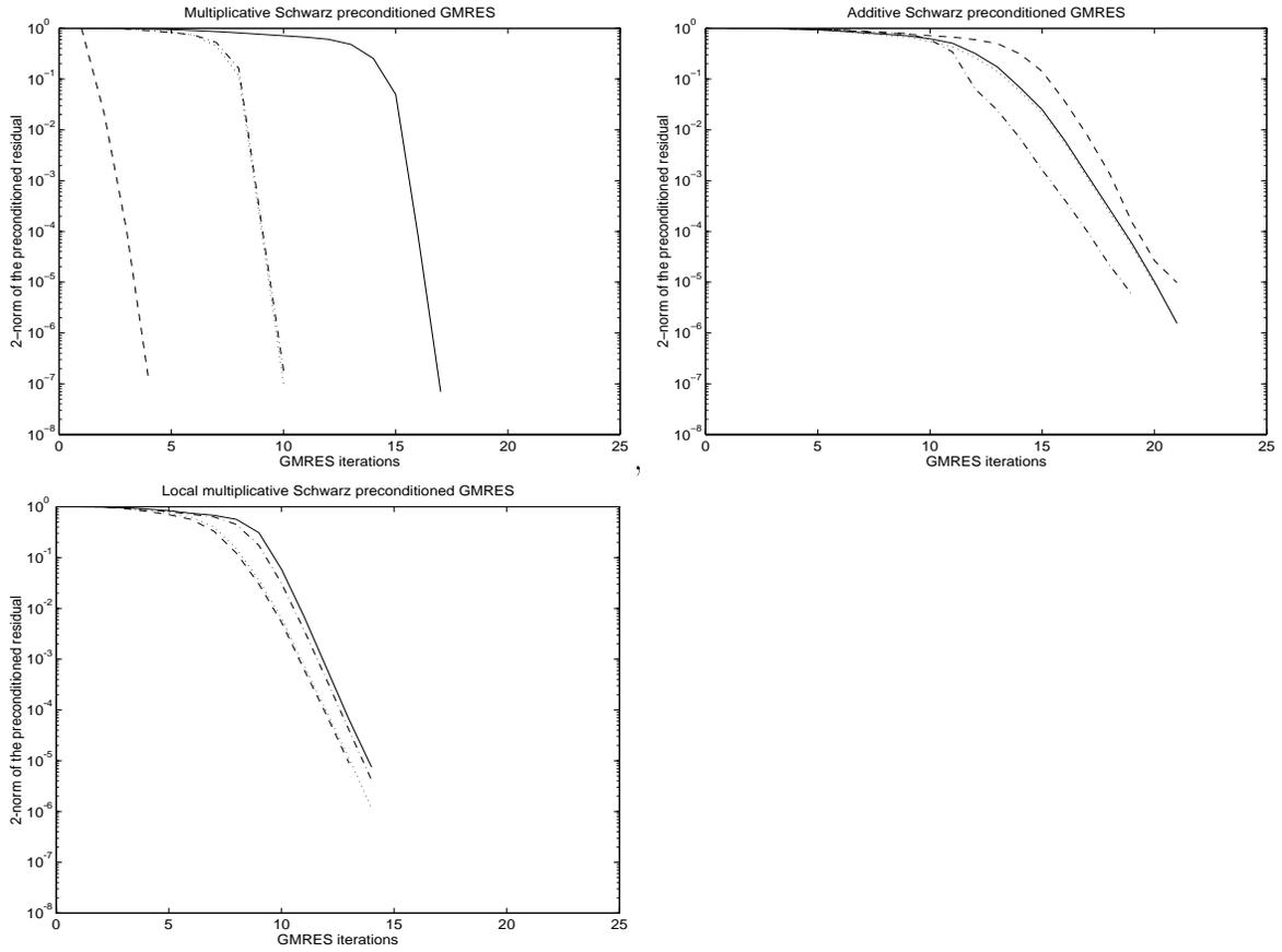
Figure 5: The figures show the iteration history of the additive (upper left), multiplicative (upper right) and the new (lower left) Schwarz preconditioned GMRES method. The line types correspond to the flow directions, i.e., solid lines  $\beta = (-1000, -1000)$ , dashed lines  $\beta = (1000, 1000)$ , dotted lines  $\beta = (1000, -1000)$  and broken lines  $\beta = (-1000, 1000)$ .
