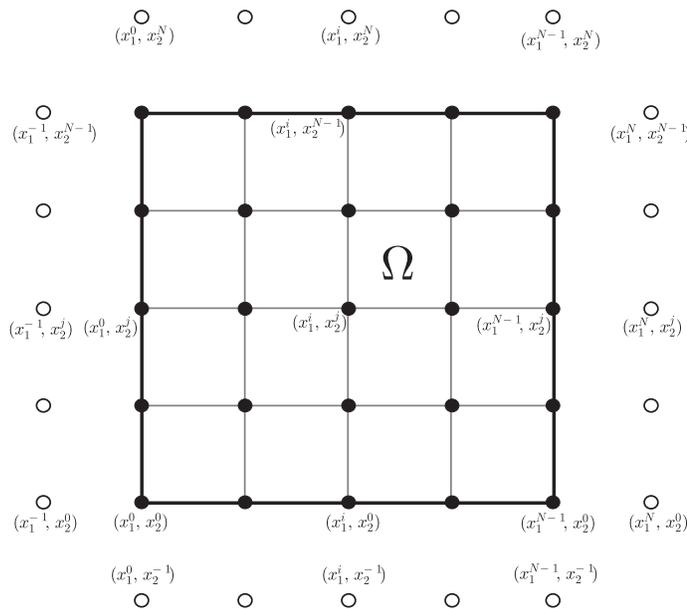
FIG. 1. Computational domain with mesh points and ghost points. Here solid circles represent the mesh points and hollow circles represent the ghost points.
