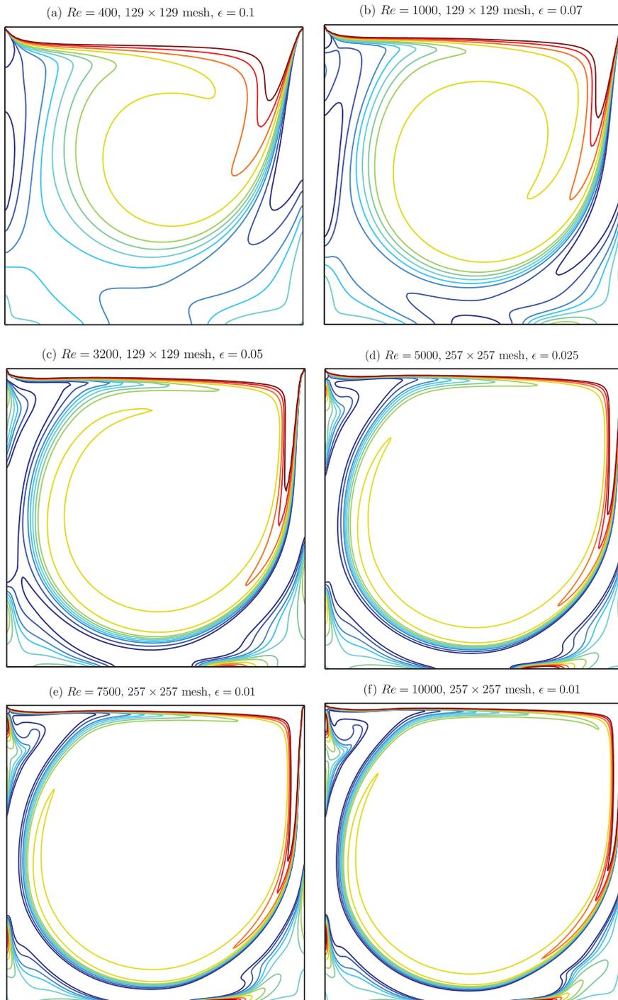
FIG. 7. Vorticity contours for the driven cavity flow problem at different Reynolds numbers.
