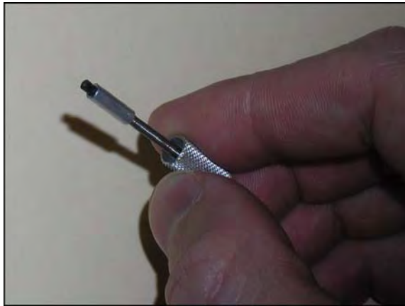
Figure 1.16 Probe installation tool with probe
