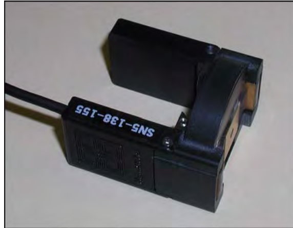
Figure 1.14 Transducer ready for probe installation
