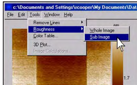
Figure 4.23 Measuring roughness within TriboView
