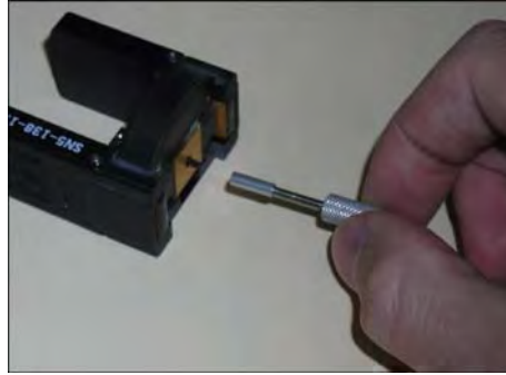
Figure 1.19 Removing the probe tool from the installed nanoindentation probe
