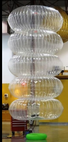
Mechanical Compression Balloon (Thin Red Line Aerospace)
