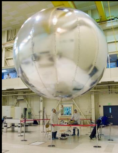
Superpressure Balloon (JPL Venus prototype)
