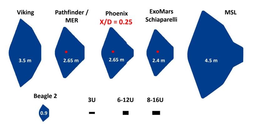
Mars entry aeroshells: blunt sphere-cone (70° half-angle)
