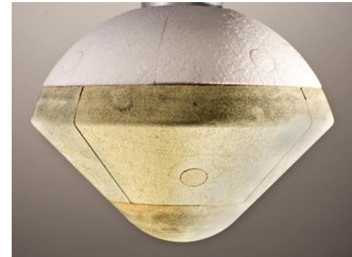
NASA Ames installed C-PICA and C-SIRCA on RED-Data2
