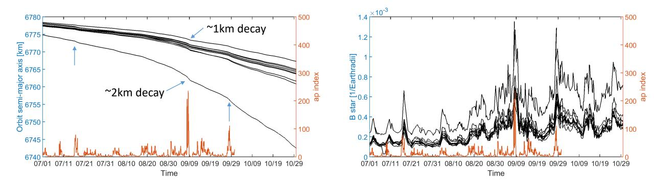
Decoupling of cross section area and atmosphere density from B\* term not easy. Atmosphere density is too variable and linked to solar activity.
