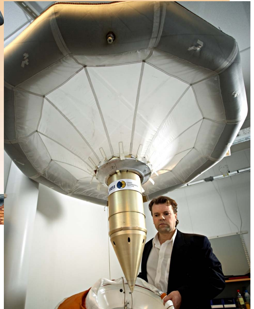
METNET : Finnish Meteorological Institute project for Mars lander/penetrator evolved from Mars-96 (inflatable skirt/ballute) architecture.
