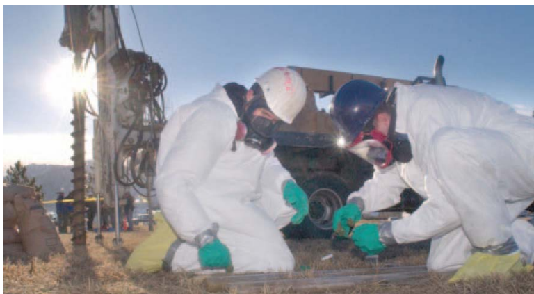
EVEN students examine a soil sample collected by hollow-stem auger drilling during the EVEN 4830 Environmental Sampling and Analysis course taught by adjunct professor Jeremy Kolenbrander.
