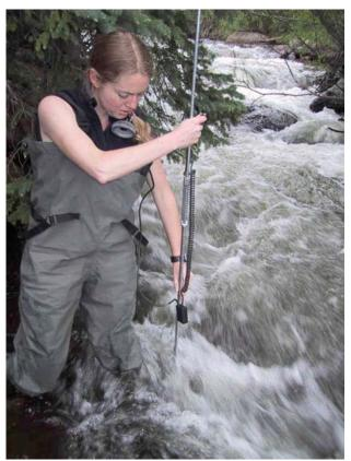
Sabre Duren, an EVEN 2002 graduate, measuring stream flow with a pygmy meter for an independent study project.
