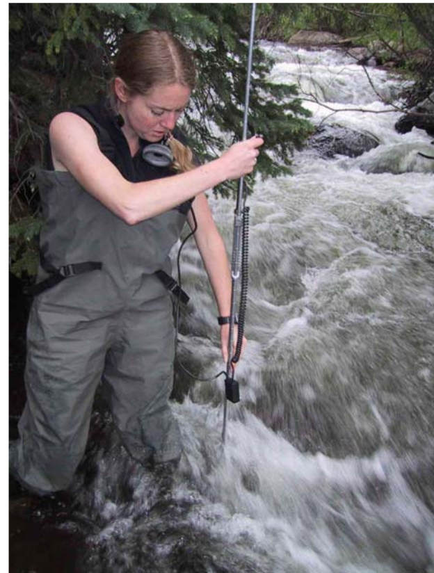
Sabre Duren, an EVEN 2002 graduate, measuring stream flow with a pygmy meter for an independent study project.
