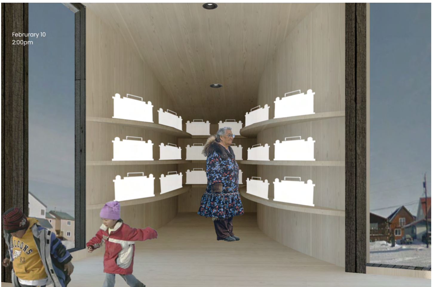
The battery wing design emphasizes features such as curved shelving for geothermally charged batteries, responding to the overall building form and a warm, as well as a wood-lined interior that creates a comfortable, clean environment. The adjacent windows illuminate the area to ensure ease of use for all generations.
