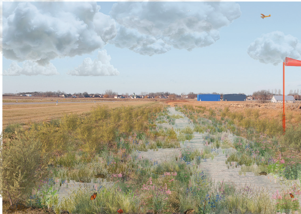
figure 55: high rainfall does not affect airport operations; swale holds water and supports a higher diversity of vegetation and some wildlife
