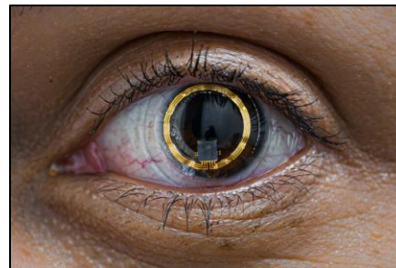
Triggerfish "smart" contact lenses monitor changes to astronauts' eyes on SpaceX's Polaris Dawn mission in September 2024.
