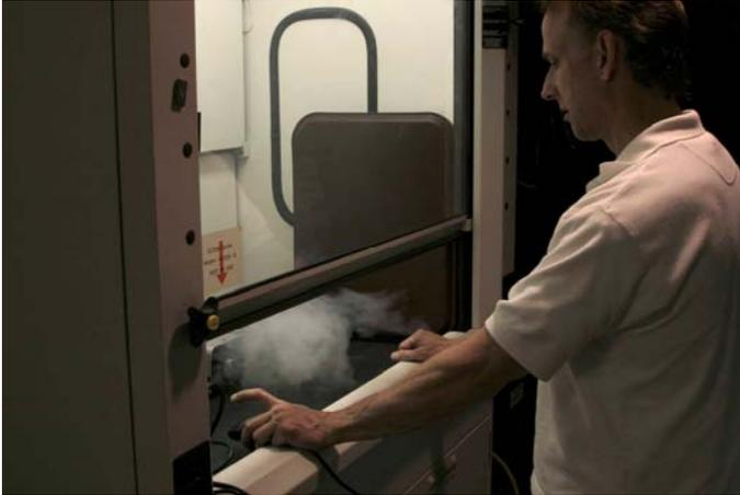
The most important decision you will make in controlling hood performance is the sash height. You have seen how the hood's performance improves as the area of the sash opening decreases. Keeping the sash at or below the safe sash-opening marker is good practice. Placing the sash at the lowest level for convenient operation will provide the best protection.
