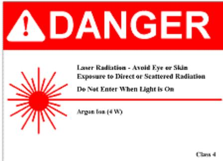
The “Caution” sign should indicate precautionary instructions, the type of laser or wavelength and the class of the laser or laser system.
