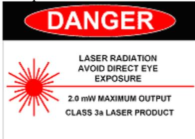
All removable protective housings will have a label affixed in a conspicuous location that conforms to the ANSI standard. The label indicates the hazard of the enclosed laser. This label does not need to contain the sunburst symbol.
