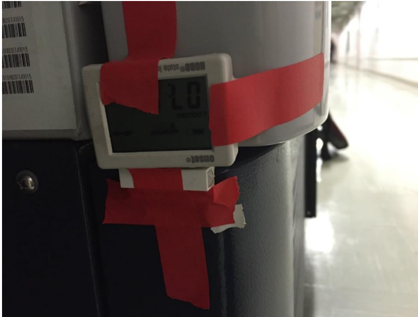
FIGURE 8: DOOR SENSOR PLACEMENT
