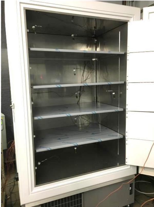
FIGURE 7: FIVE COMPARTMENT FREEZER VIAL PLACEMENT
