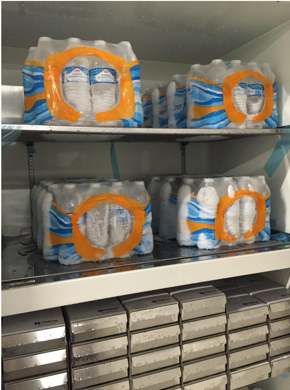
FIGURE 15: ULT FREEZER FILLED WITH WATER
