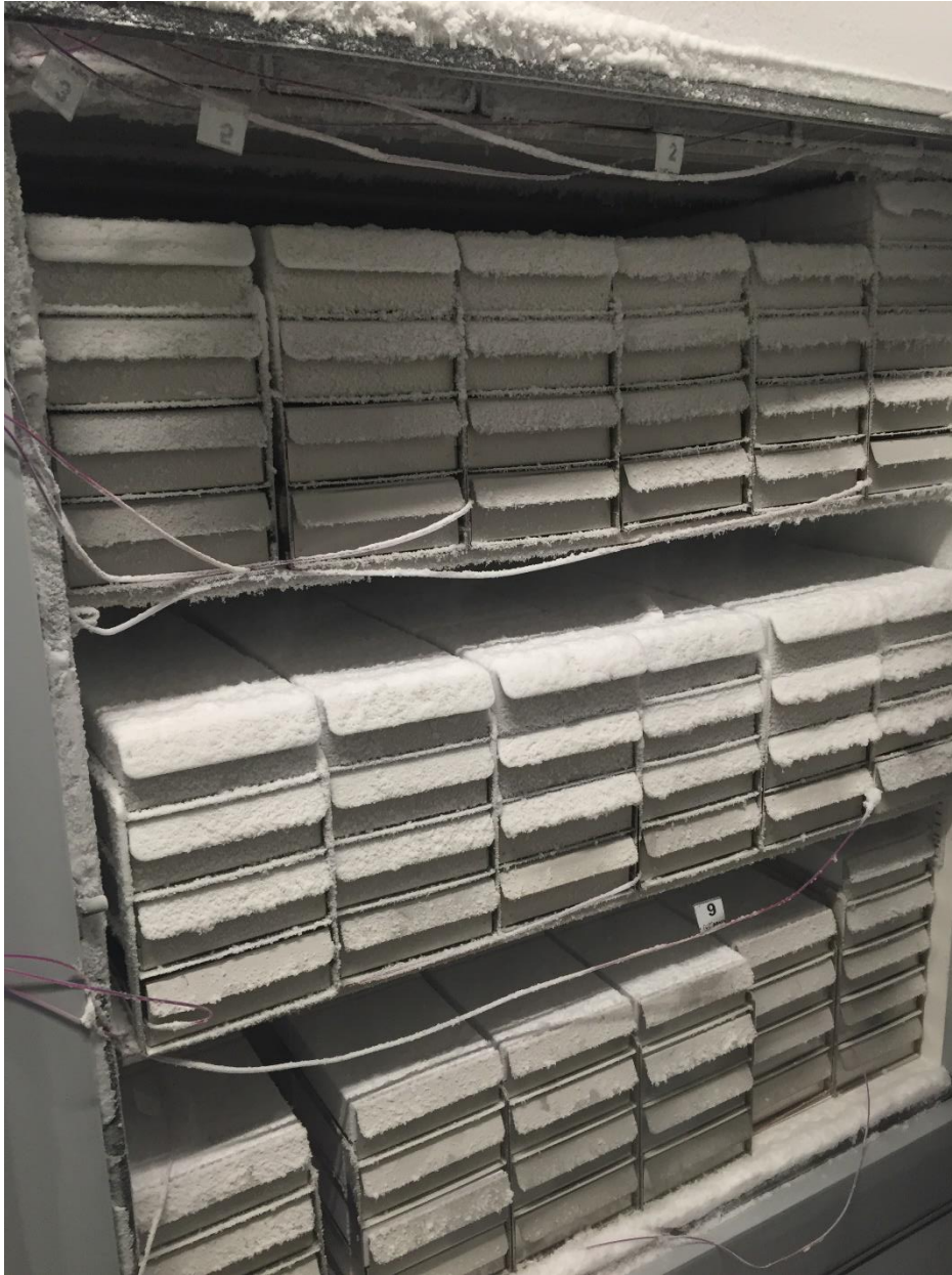
FIGURE 14: THERMOCOUPLE PLACEMENT IN FULL ULT FREEZER
