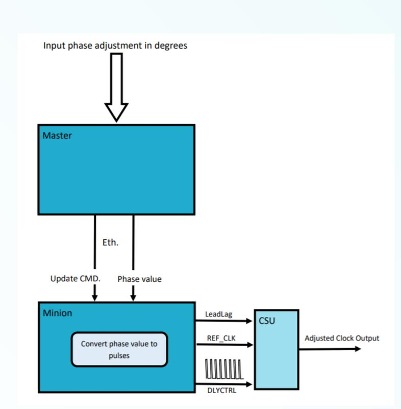
Figure 2. NNTS Functional Diagram
