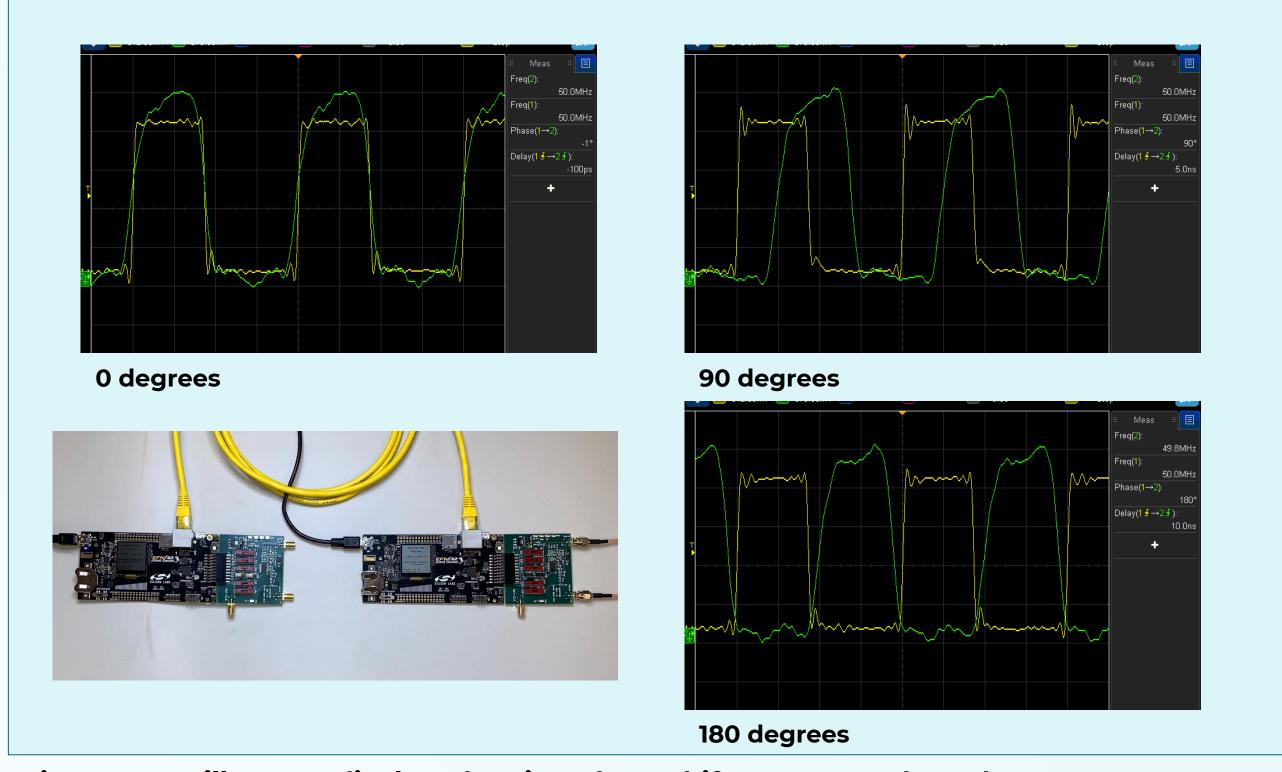
Figure 3. Oscilloscope display, showing phase shift at 0, 90, and 180 degrees
