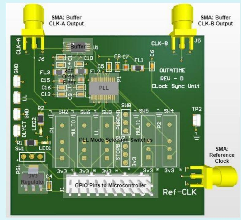
Figure 4. Clock Synchronization Unit (CSU)
