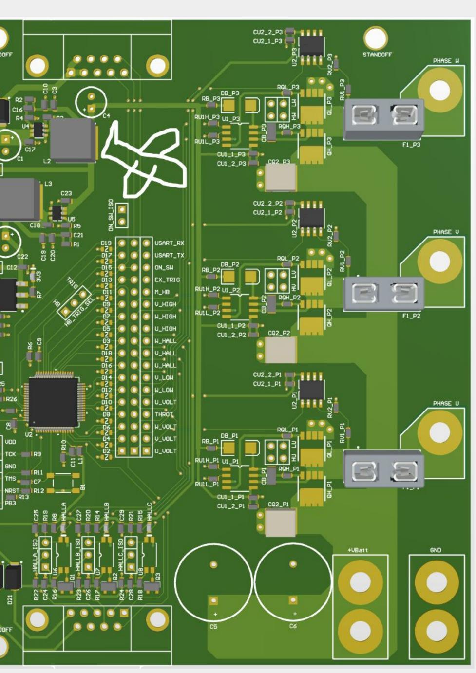
**Figure 6:** Motor Driver Module (MCU/MCU Power)
