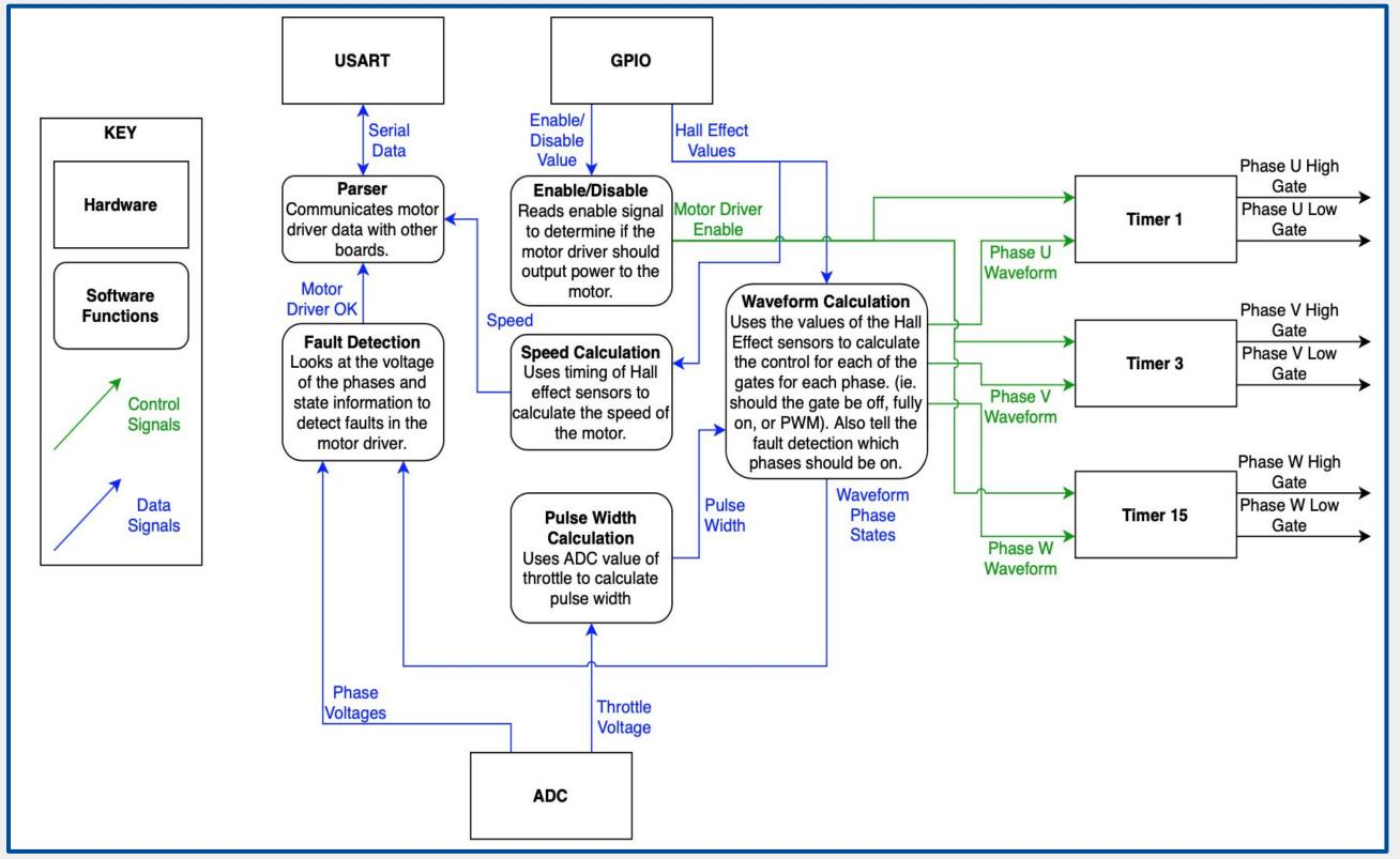
**Figure 3:** Motor Driver Software Flow Diagram
