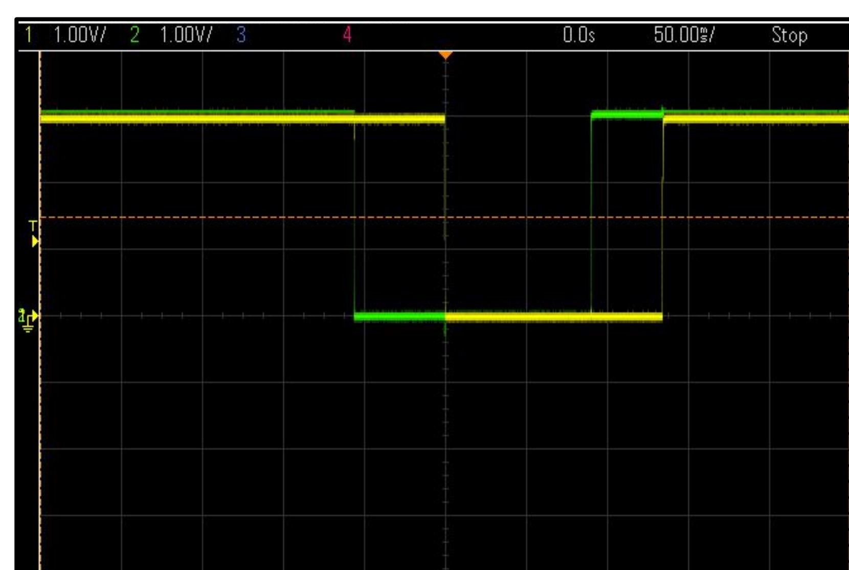
Oscilloscope measurement of falling edge from hall effect sensor
