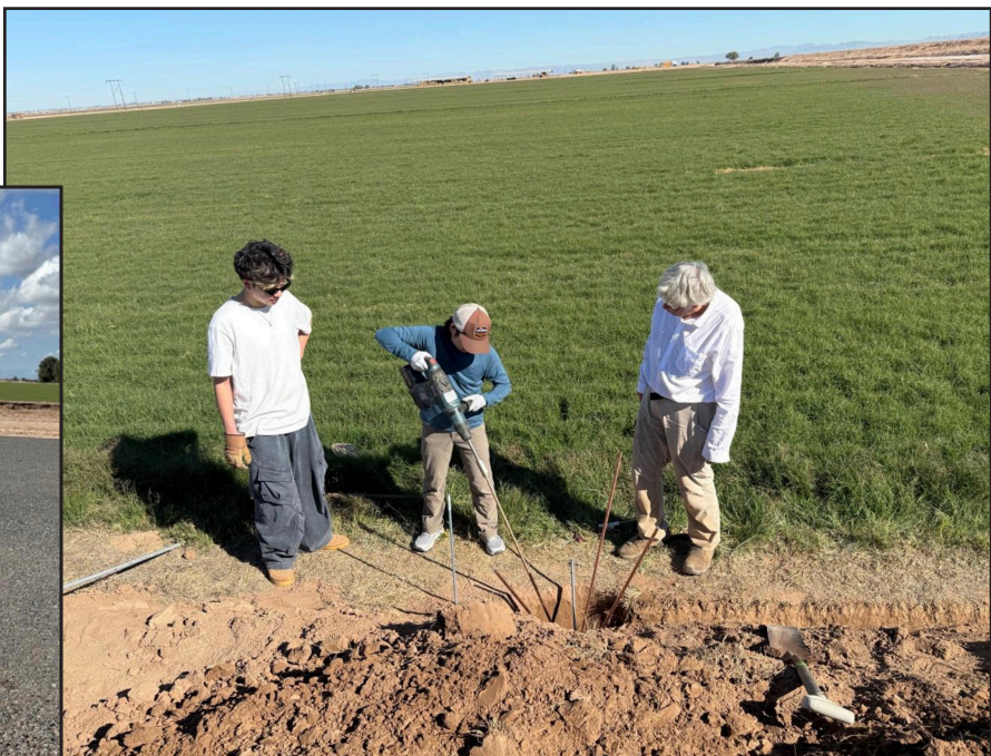
Graduate students Morow Tan and Hong-Mao Huang and professor emeritus Roger Bilham install a creepmeter across the Brawley fault. The students use an impact hammer to drill rebar rods into the soil, which serve as anchors for the two ends of the creepmeter instrument. photo credit: Kathryn Materna
