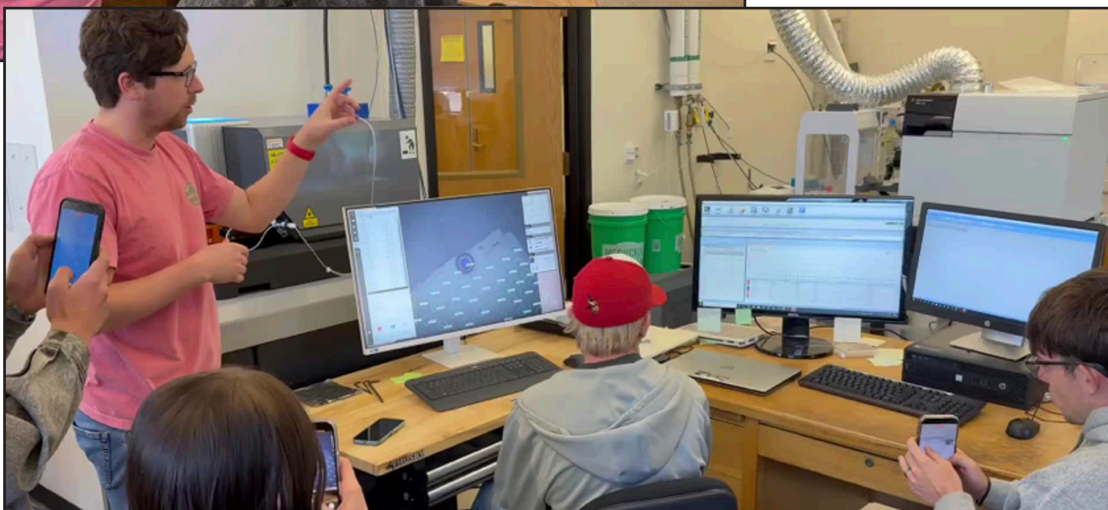
Dr. Cullen Kortyna hosting Northglenn high school students in TRaIL during acquisition of detrital zircon U-Pb geochronology for the Tava sandstone, a Snowball Earth-aged unit in Colorado. Here Cullen explains the process of setting spots on the zircon for U-Pb dating.
