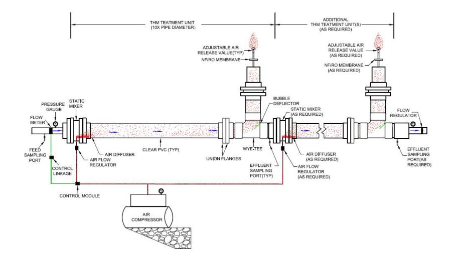
Figure 4.3 Layout of Horizontal Pilot-Scale Diffused Aeration Apparatus
