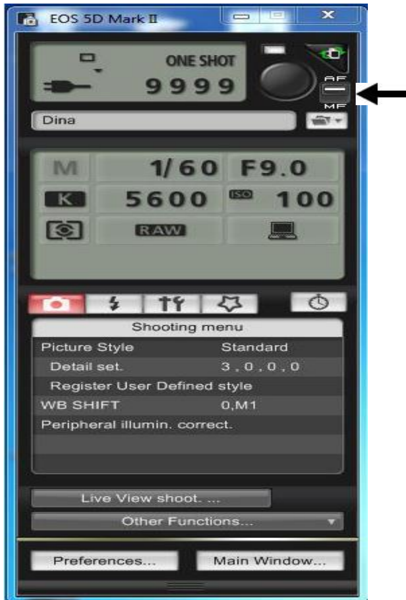
Figure 17. If the camera has a focus failure it will need to be tricked into capturing the image. To do this, place a dime at the center of the sheet and hover over the shutter and switch the focus from auto to manual. Remove the dime and capture the image.
