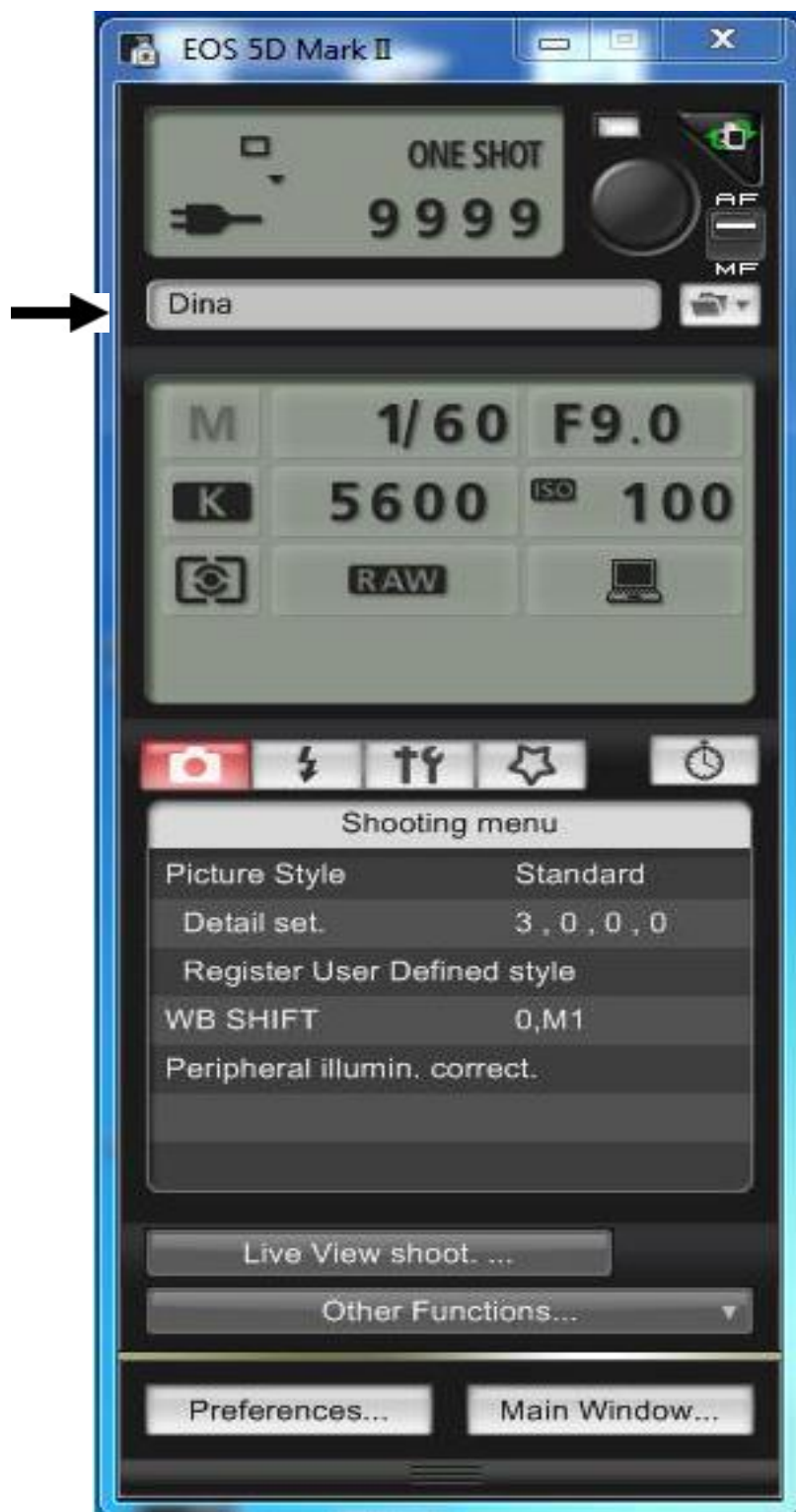
Figure 3. If the folder pathway is selected correctly your name will appear under the shutter shown with the arrow above. If your Identikay name appears here images are not being stored to the public pictures area and will not be available for post processing.
