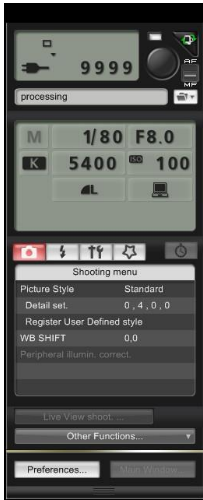
Figure 3. Very dark and very bright washed out images do not OCR well. COLO uses the settings above to create a balance between the two extremes and seems to produce images that OCR well.
