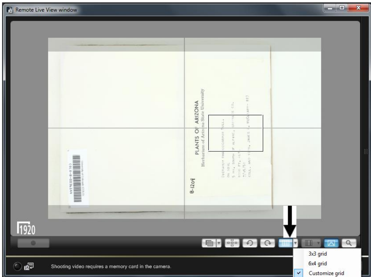
Figure 2. Using a custom 2 x 2 allows the imager to quickly find the center of the image and allows the use of the grid to assure the fold of the packet represents the center of each image captured.
