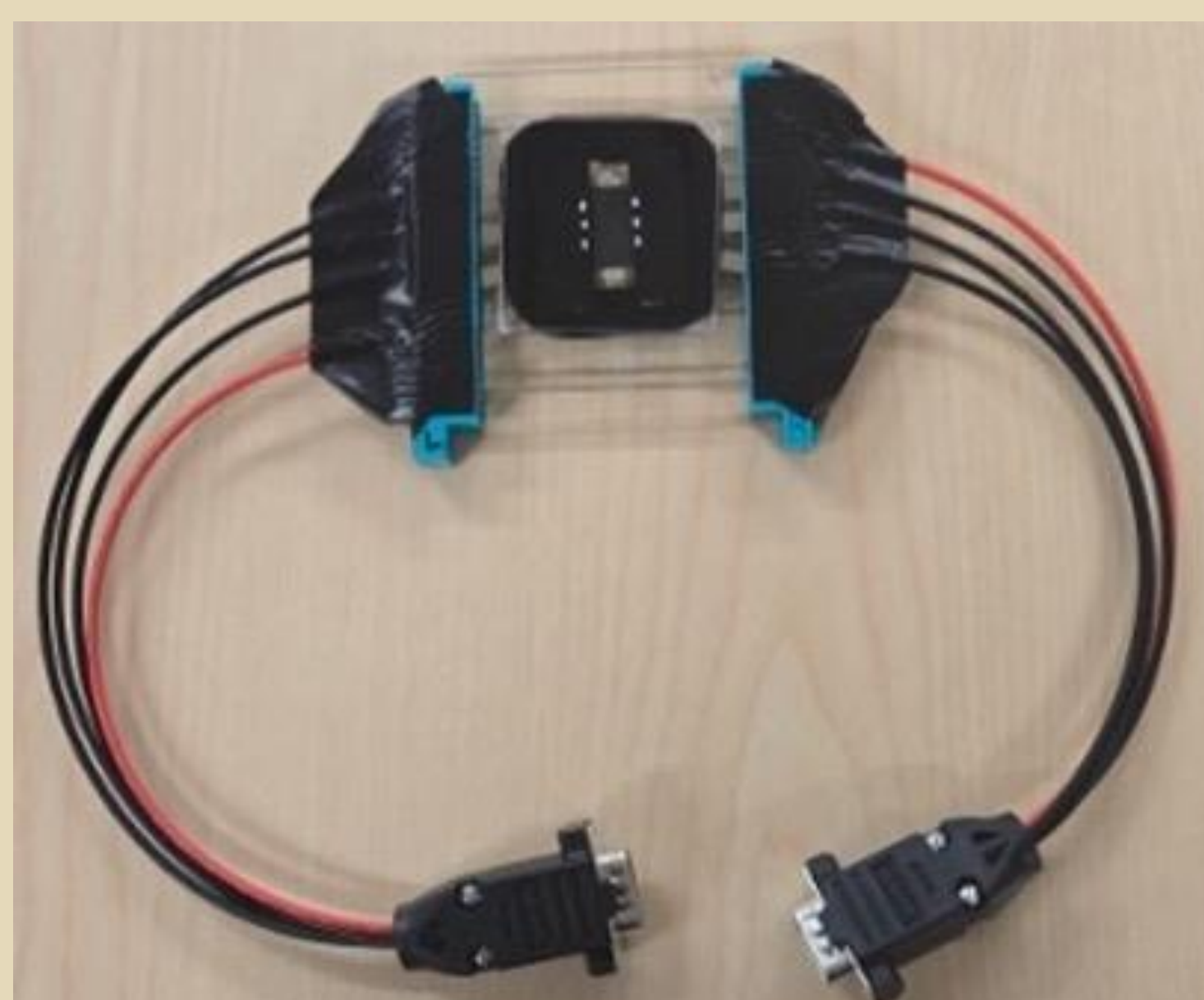
Example of solar cell. Six white dots in the center of the cell packaging are guides to indicate location of pixels.
