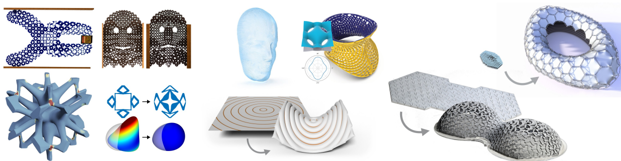
Figure 1 Examples of structures whose design we will study in these lectures. From left to right: metamaterials designed to emulate continuum elastic materials ([59, 39, 64]); surface-based inflatable structures that deploy into a programmed shape [41, 46] upon inflation; and two deployable structures based on bistable auxetic metamaterials and Hoberman-sphere type mechanisms [12, 45].
