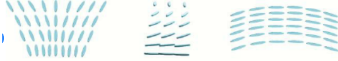
Figure 9. Splay (left), twist (center) and bend (right) deformations of the director field.
