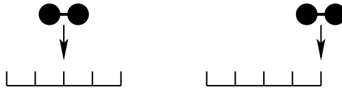
Figure 7.4: Changes in the empty interval probability E_m for m = 4 , with an adsorption event in the interior of the interval (left) and at the edge of the interval (right).
