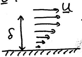
velocity profile in laminar flow near a boundary. There is a boundary layer of thickness  $\delta(Re)$  which governs how far away from the boundary the effect of the boundary causes the  $v$  to deviate from  $U$ , the velocity far from the wall.
