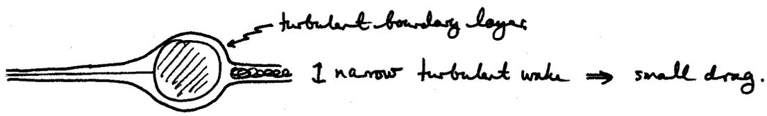
Hence the turbulent wake is narrower, there is less "sucking" and so there is less drag than when there was a laminar boundary layer. The drag crisis is a result of the boundary layer becoming turbulent.
