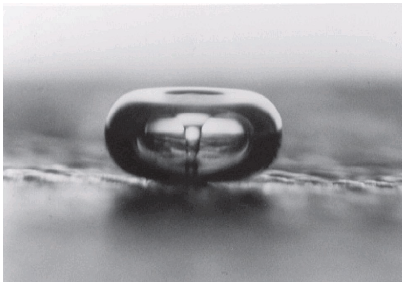
Figure 6. An asymmetrically collapsing bubble next to a wall. The bubble formed in water that was shaken at a frequency of about 60 Hz with the ambient air pressure near the liquid's vapor pressure. The maximal diameter of the bubble is about 1 mm. (Photo from L. A. Crum, Journal de Physique Colloque 40 , 285, 1979.)
