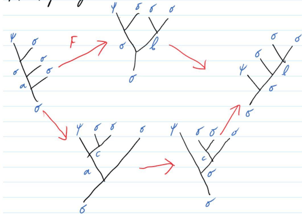
For consistency, different  $F$ -moves need to get us to the same diagram. This leads to the **pentagon equation** — the only consistency condition which involves exclusively changes of basis. Let us write the consistency equation for  $F$ -moves for the two different paths in F17:
