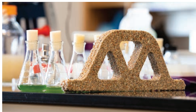
Prometheus Materials, formed by CU researchers, uses living microalgae to make bio-cement.
