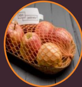
**Packnatur Tube Netting:** *(screen material)* a material made from beechwood cellulose and 100% plant based biopolymers with all natural dyes - used in sustainable food packaging
