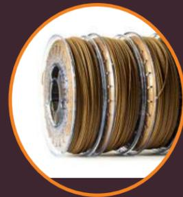
**Hemp 3D Print Filament:** *(used to create all cultural container bins and monuments)* a closed loop material made from PLA and hemp that prints at low temperature with no odor- the material can be painted with VOC free plant based dye
