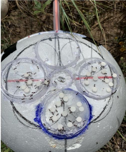
Figure 6: Payload infested with ants due to lack of hot glue surrounding the glass slides, E.coli, and the lids of the Petri dishes used to form a secure adhesive.
