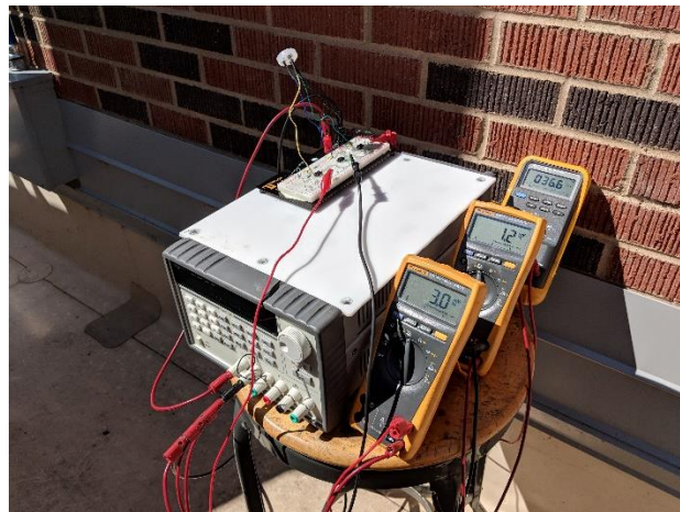
Figure 22. Electronic testing on breadboard, UV sensor array.
