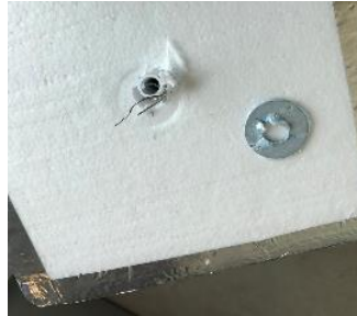
Figure 19. Damage inflicted by stair test.
