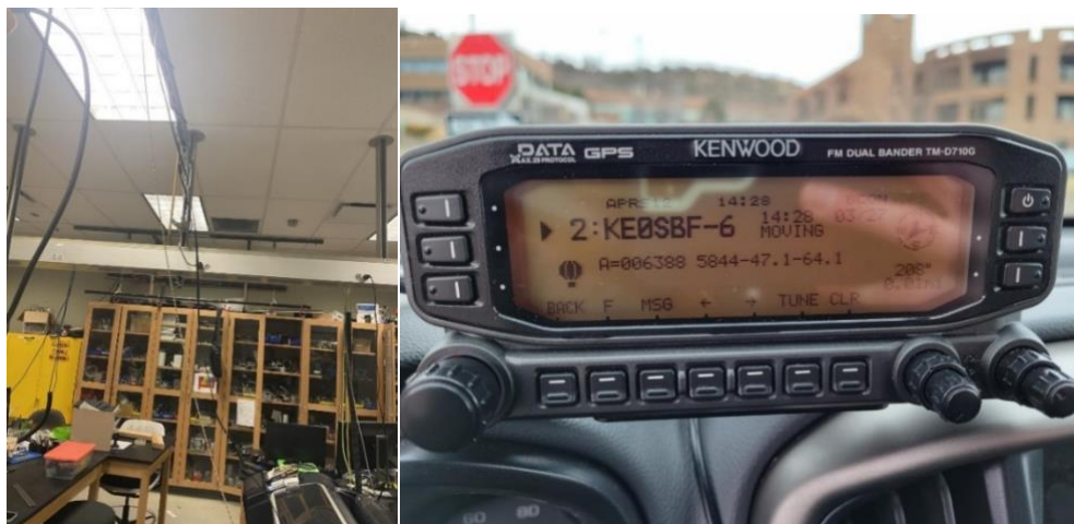
Figure 6: Left: Antenna hanging up during initial comms test. Right: APRS traffic decoded by mobile ground station, showing GPS altitude and example voltage, internal, and external temperature data.
