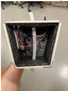
An image of the arduino being housed in the payload
